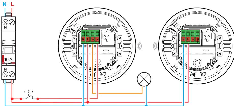
The master can be paired with a maximum of 5 sensors configured as slaves.
